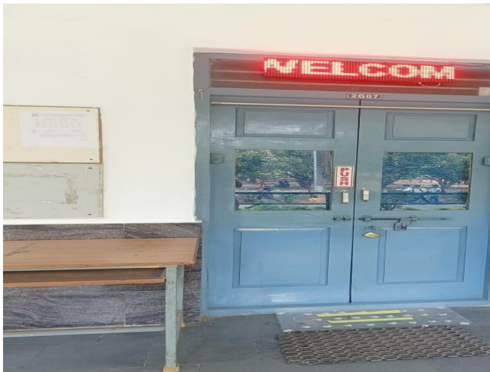
Fig 7 : LED Digital display by using footstep power generation
