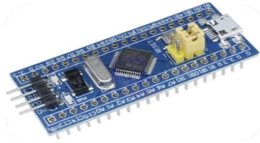
Fig 2 : STM32 ARM Cortex-M3 Series Sensor Interfacing and Data Acquisition
